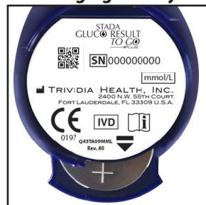
Turn Meter over until the Meter label is facing up. Look for Battery Tray symbol on Meter label and pull Battery Tray out until battery is exposed. Replace battery.
